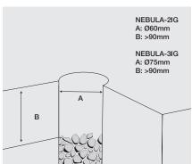
1. Prepare opening on concrete surface with gravel beneath for drainage.
